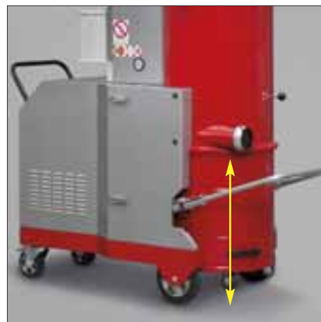
Progressive lowering of the collection bin
